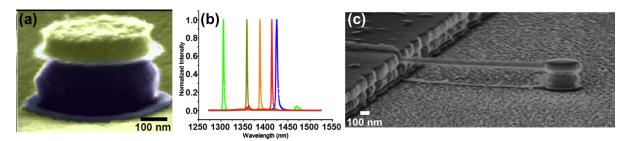
Fig. 2. In (a), we show an SEM image of a fabricated nanopatch laser. The device has the smallest physical volume for a semiconductor laser. In (b), we show lasing spectra for various device radii. In (c), we demonstrate a method to contact the top patch with a thin gold wire for electrical injection.
