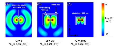
Fig. 1. In (a), (b), and (c) we show the successive reduction in radiation for a 500nm x 400nm x 200 nm semiconductor block by introducing a reflective metallic box around it. Using metal, we can achieve quality factors as high as Q = 3100.
